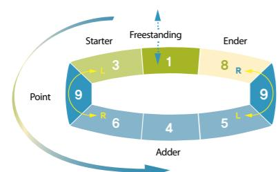
The freestanding module is only used when needed with the enclosed layout.
